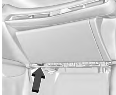
Interior Power Outlet
